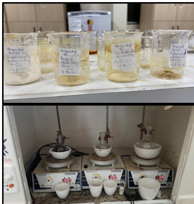
Figure 1. Experimental setup for synthesis and crystallization of BZD.
